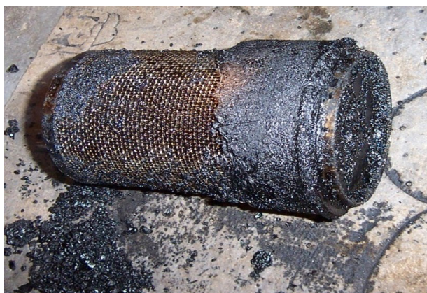
Figure 3. Severe build-up of solid carbon.
