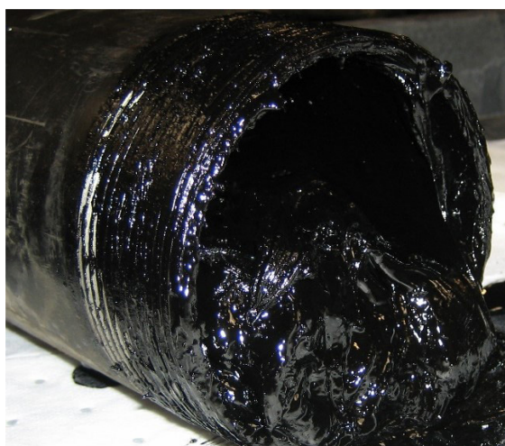
Figure 2. Thermal fluid sludge.
