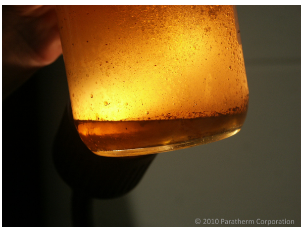
Figure 2. Water will quickly manifest itself in high temperature thermal fluid systems. If water does get in the system in an appreciable concentration, it can only be removed with a controlled boil out procedure.
