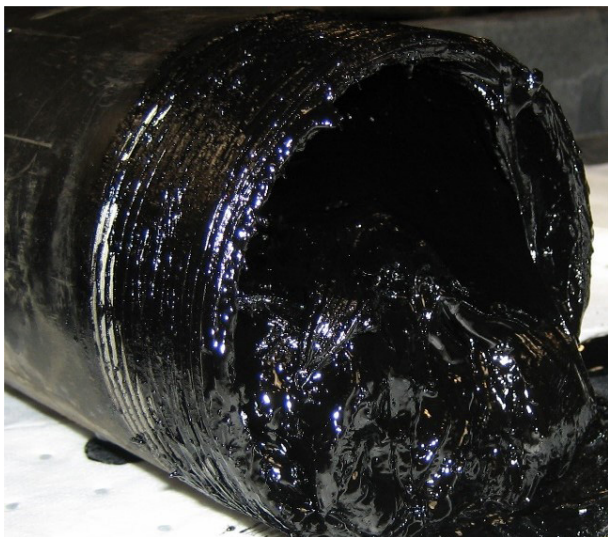
Figure 1. Sludge is formed over time as oxidation byproducts accumulate. Sludges are a significant detriment to performance, and often can shut systems down. Oxidation is eliminated with inert gas blanketing, or otherwise thwarted by filtration or reducing expansion tank temperatures.
