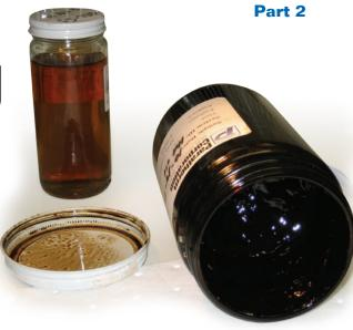
FIGURE 1. A very high viscosity thermal fluid can be a reason for failure of a heat-transfer system
