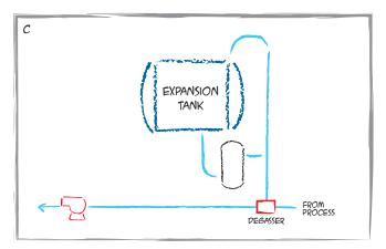
**Exposed tanks** — It's not a good idea to paint an expansion tank black if it is located outside in the sun. Light colors or silver should be used to reflect the sun light. Even better is to install a sun shield.
