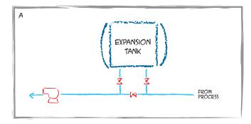
make sure the 2nd line (farthest away from the pump) is closed off once the oil temperature is >275°F. If there is a valve on the expansion line, it should be 2/3 closed to minimize thermal currents into the tank. This valve should never be completely closed during operation.
