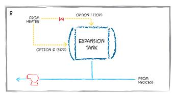
important to make sure that the valve is closed before the heater outlet temperature exceeds 250°F. The tank may not appear to be hot because the flowrate through the usually small diameter (<2") line is not enough to heat up the entire tank. But oxidation will occur because the fluid flowing into the tank will be at the heater outlet temperature and will thoroughly mix with the air in the head space.
