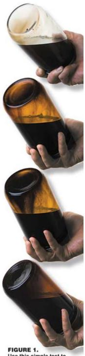
Use this simple test to find the degree of carbon contamination in your thermal fluid extremely fine carbon particles (soot) that can agglomerate to form sludge deposits.
