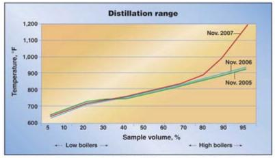
FIGURE 3. The second annual test (Nov. 2007) shows why periodic testing is important; contamination or oxidation resulted in a dramatic increase in high boilers
