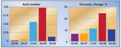
FIGURE 2. Key fluid parameters, such as acid number and the change in viscosity, should be consistently recorded to track discrepancies and overall trends in fluid behavior over time
