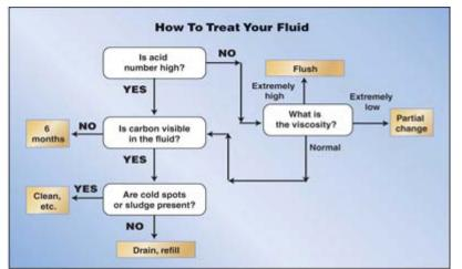
FIGURE 4. Solutions to common thermal fluid problems can be found by analyzing the results of a few simple tests
