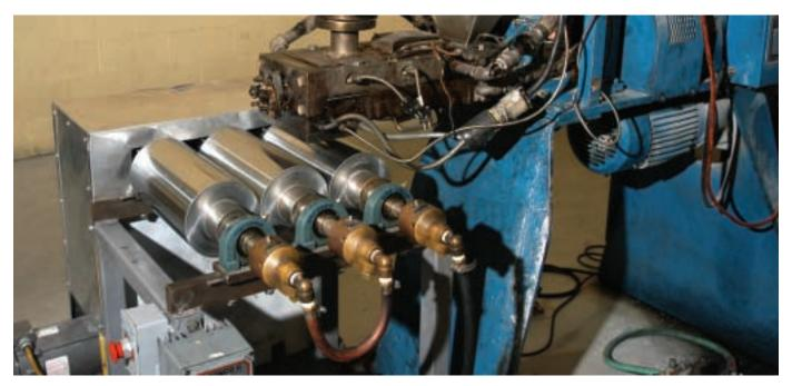
Readco Continuous Processor Barrel Extruder equipped with Three Roll Sheet Stack. Temperature controlled with Paratherm heat transfer fluid.
