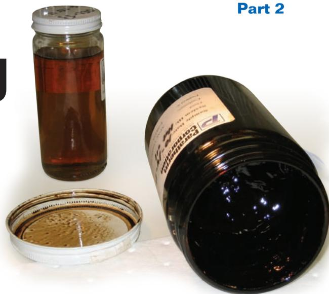
**FIGURE 1.** A very high viscosity thermal fluid can be a reason for failure of a heat-transfer system
