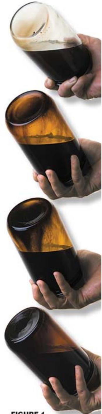
**FIGURE 1.** Use this simple test to find the degree of carbon contamination in your thermal fluid
