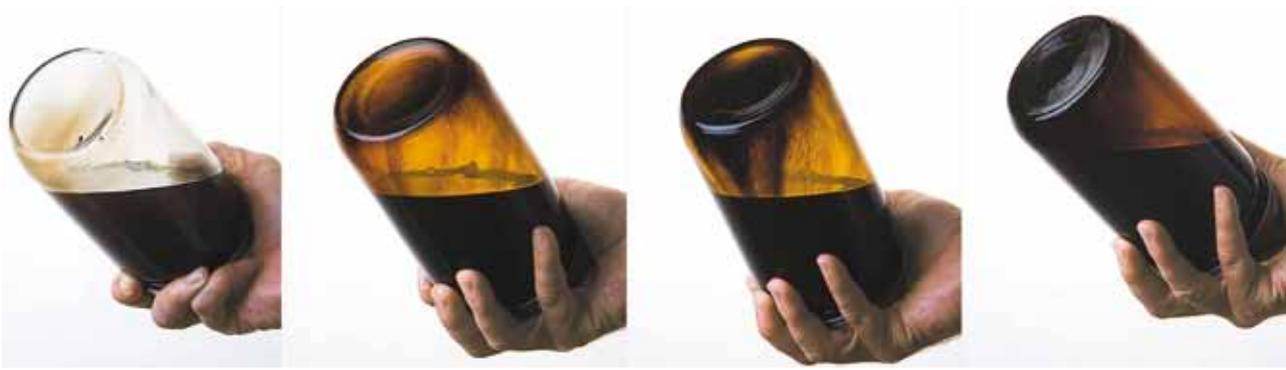
**Figure 1.** Viscosity, consistency and colour of fluid will vary with age and use conditions; dark colouration does not necessarily reflect poor fluid condition, so although visual inspection can provide clues, it is always best to verify with lab analysis.
