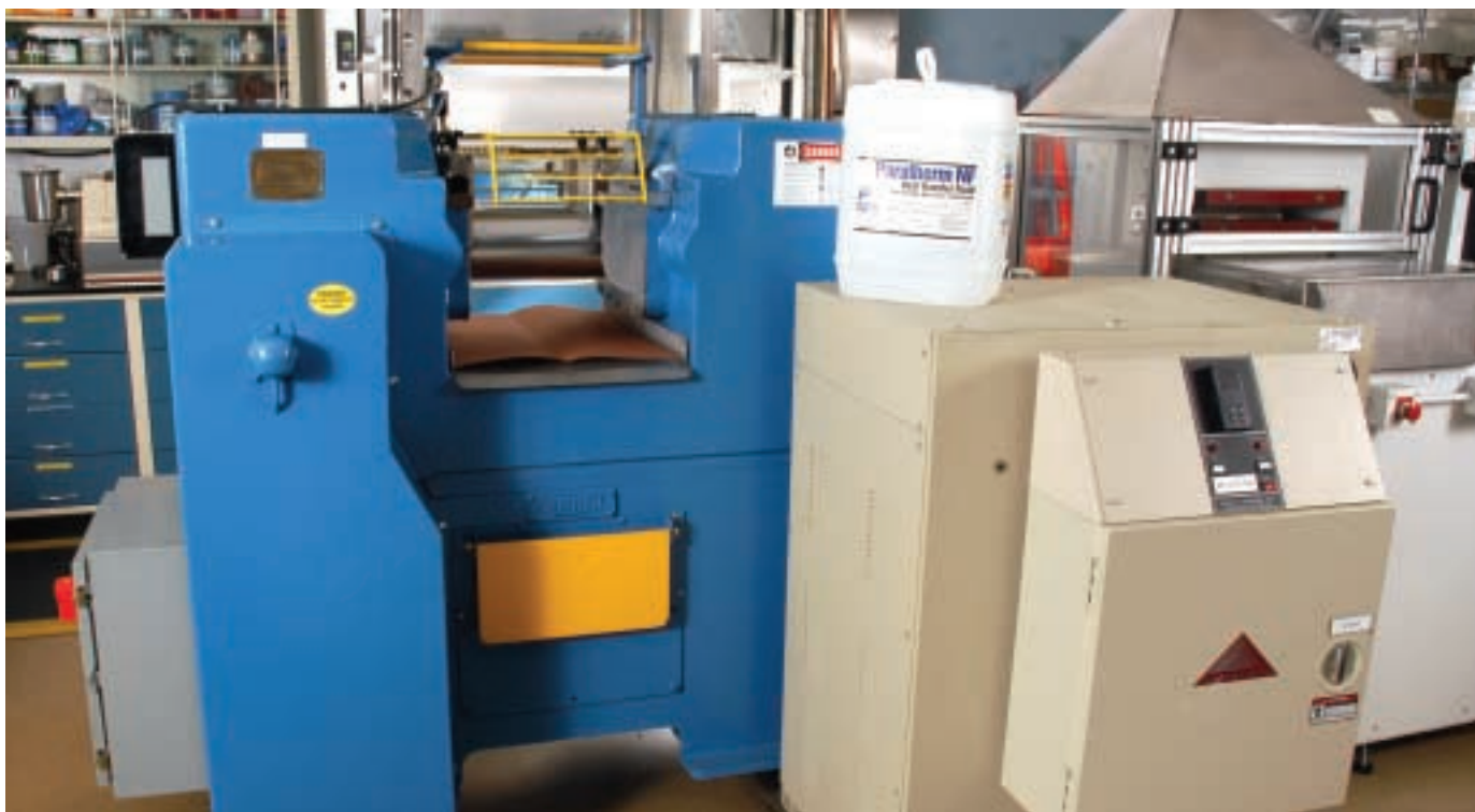
The rolling mills at AGC Chemicals America are used to compound the fluoropolymers that are an essential component in certain data cables and other wire and cable applications, as well as automotive and industrial seals and gaskets and down-hole oil and gas applications.
